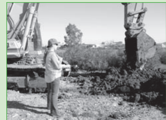
Above: Monitoring VOC levels in the air where excavations are occurring with a photo-ionisation detector.
