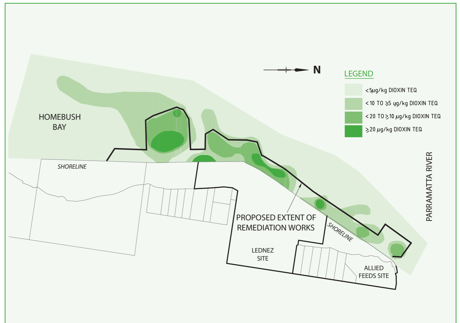
Above: Drawing showing the newly approved Homebush Bay sediment remediation area – 45% larger than before.
